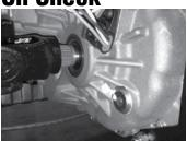
The level check/fill plug is located on the back, passenger side of the gear case. Maintain the oil level even with the bottom of the level check/fill plug hole threads.
