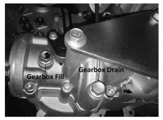
The drain plug is located on the lower passenger side of the gearcase.
