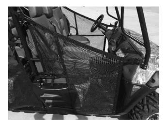
**DANGER:** Falling from a moving vehicle could result in serious injury or death. Always fasten your seatbelt and secure the safety cab net.
