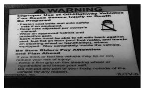
Seat belt and Safety Warning – Located on vehicle firewall.
